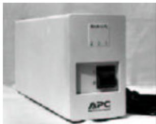
**Energy Absorption/Dissipation:** This tells you how much punishment the unit can take before failing. The rating is measured in joules and you want a high number. Most homes can get along with a rating of 200 to 400 joules. Units which can absorb 600 joules or more tend to be expensive, but they are worth the money if you need the protection.
